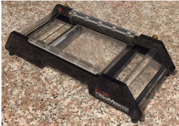
Figure 4.1. Submarine gel electrophoresis tank for running agarose gels.
