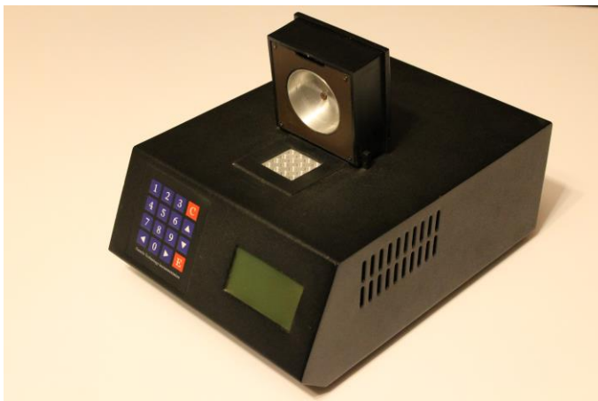
Figure 3.5. A typical DNA thermal cycler has a heating block, heated lid, keypad and an LCD display.
