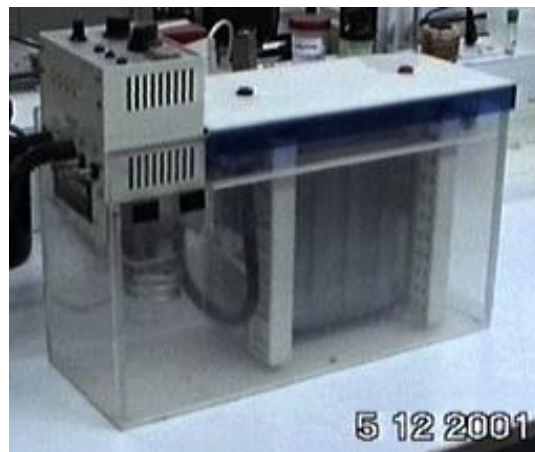
Fig. 5.4. Apparatus for denaturing gradient gel electrophoresis. The main buffer compartment contains an immersion heater and a buffer circulation pump that maintains a constant temperature of 60°C throughout the electrophoresis run.
